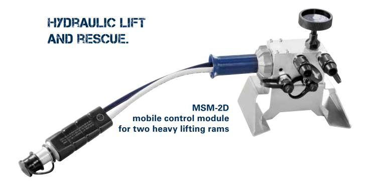
One motor pump, two applications. If loads have to be lifted during a rescue as well as using cutters, spreaders and rescue rams, then the patented MSM-2D allows two heavy lifting rams to be connected to the power unit. For example, this may be to lift trams, underground trains, trucks, buses or trains involved in accidents. Heavy lifting gear is also used during rescues in collapsed buildings.
