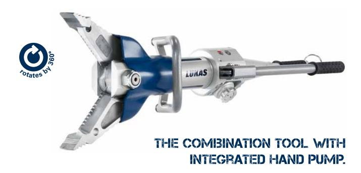
The SC 250 M combination tool with built-in hand pump is the affordable entry point for rescue work. It is completely self-sufficient – without power unit, hose or cable. It is instantly ready for use, it can cut and spread without modifications, and is especially suited to rescues in areas at risk of explosion (no sparks), in rough terrain and for equipping rescue helicopters or technical rescue.
