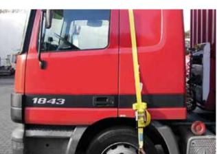
As the suspension of modern trucks' driver cabs often has a negative effect on the state of the injured, rescuers have to minimise the cab's movements. To do that, LUKAS provides a special cab safety kit which can be universally used. It is hooked in on both sides to the holes in the wheel rims and is then tightened with a ratchet or is fixed with a loop around the front axle. WEBCODE: Imqusz
