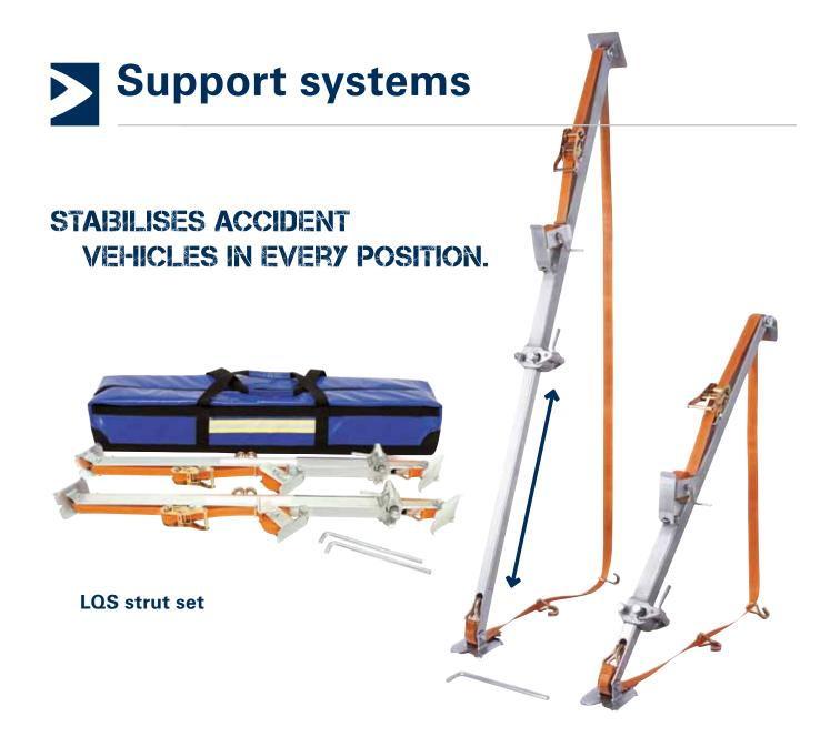
For more safety the struts are applied diagonally at an angle of 25° to 35°, they are attached to the vehicle bodywork with hooks and are jacked up with a ratchet. It is very quick and easy to manually adjust their length. The complete set consists of two props (adjustable from 48 to 78.7 in. / 1.22 m to 2 m) in a carrying bag.
